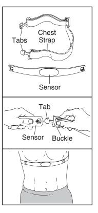
attach the other end of the chest strap to the sensor. Adjust the length of the chest strap, if necessary.
